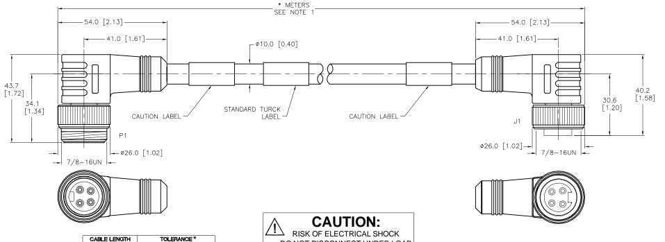
WHICHEVER IS GREATER STRIP LENGTH TOLERANCE\* 0-7mm ±0.5mm 8-29mm ±1.0mm 30-49mm ±2.0mm 50-69mm ±3.0mm 70-100mm ±4.0mm NOTES: \*UNLESS OTHERWISE SPECIFIED
